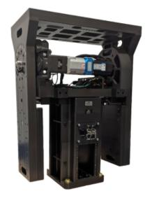
The QLA-360MPT-90 is a modular positioner designed for Low Earth Orbiting (LEO) tracking satellite applications. The modular construction consists of eight sub-assemblies (not including counterweights) with the heaviest sub-assembly weighing less than 130 lbs. The positioner can be fully assembled with two people in less than 2 hours.
