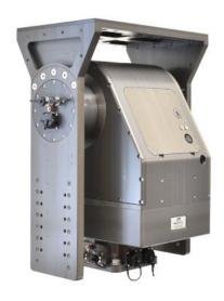
The QLA-360FER-55 is a Power Over Ethernet (PoE) antenna positioner designed from the ground up to automatically point and peak directional antennas for microwave Line of Sight and satellite communications. Satellite applications include geo stationery positioning and inclined orbit tracking.
