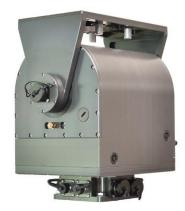
The QLA-360MPT-30 is a Power Over Ethernet (PoE) antenna positioner designed from the ground up to automatically point and peak directional antennas for microwave line of sight or satellite communications. The LinkAlign-360MPT-30 is intended for continuous tracking applications.
