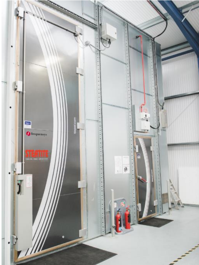
Fig. 1. View from outside our Spherical Near-Field Range.
