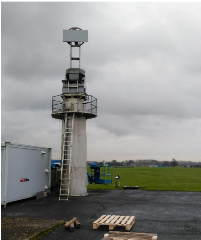
Fig. 8. Planar Array Antenna mounted on the Independent Far-Field range
